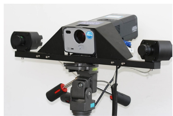
Figure 1 Structured-light 3D scanner. The device consists of two charge-coupled device cameras and one projector.
