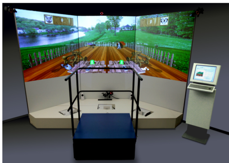
Figure 7 STABLE, a platform with diagnostic facilities and training programmes, mainly focused at stability training.
