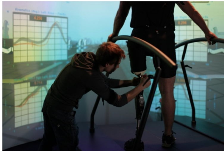
Figure 6 GRAIL, a treadmill, combined with a screen on which a scenario is projected and performance of the patient is required.
